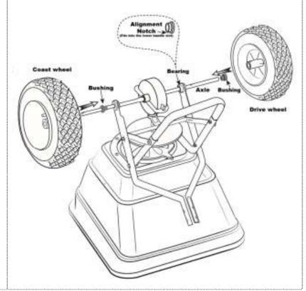
**Step 4:** Install COAST WHEEL onto the AXLE fully, then using outside Cotter Pin hole, insert 1" Cotter Pin through AXLE (not thru the wheel). Bend with pliers to prevent pin from falling out.
