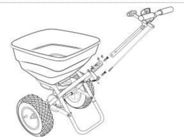
**Step 7:** Remove one 1/4-20 Hex Nut from the CONTROL ROD. Next, push LEVER forward to setting "0" to help align the CONTROL ROD with hole in PIVOT BRACKET, pull LEVER backward to insert CONTROL ROD through hole in PIVOT BRACKET. Now install 1/4-20 regular nut on to CONTROL ROD.
