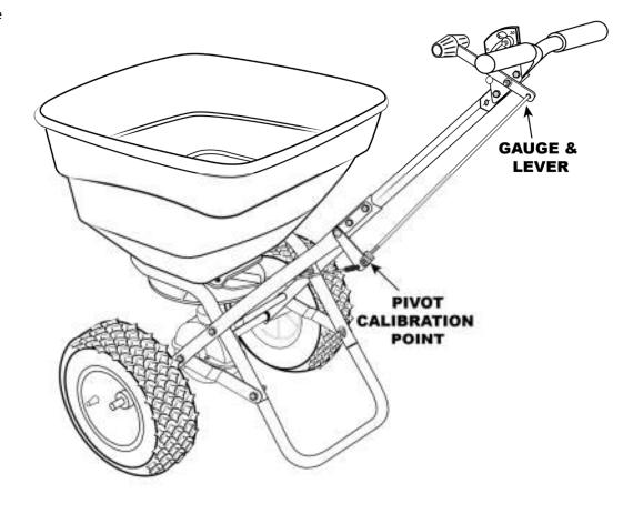
below. *TIP:* If your shut-off is not able to **OPEN** fully, loosten the bottom nut a few turns, then tighten the upper nut so that it allows you to push the **shut-off fully open**. Next, tighten each nut so that they contact the PIVOT BRACKET without moving it.
