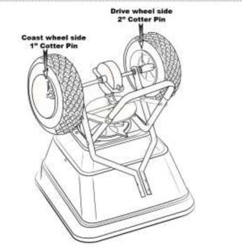
**Step 5:** Now remove the PIVOT BRACKET from THE LOWER HANDLES. Keep the 1/4 -20 x 2" bolts and locknuts for use in reinstallation.
