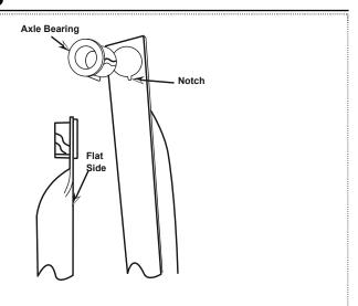
**Step 3:** Install DRIVE WHEEL onto the AXLE and align with the Cotter Pin hole nearest to the LOWER HANDLES as shown. Insert 2" Cotter Pin through WHEEL and through AXLE. Bend with pliers to prevent pin from falling out.
