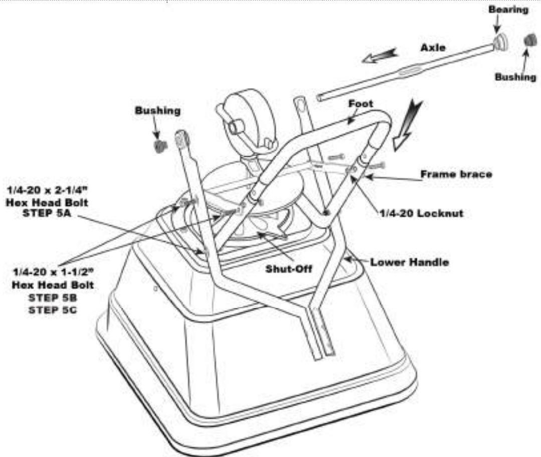
**Step 6:** Places the bearings into the lower frame using the “notch” on the bearing to fit into the “notch” on the LOWER AXLE FRAME. Next slide the axle through the bearings, through the GEAR BOX and into the other LOWER AXLE FRAME. Next, install AXLE BUSHING onto the axle, by placing the smaller end in first, slide over the AXLE, past the drilled holes.
