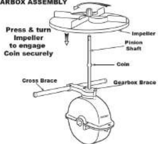
**Step 4:** Install GEARBOX by inserting the PINION SHAFT into hole in center of HOPPER bottom. The word "FRONT" on the GEARBOX must point to Front of the HOPPER.
