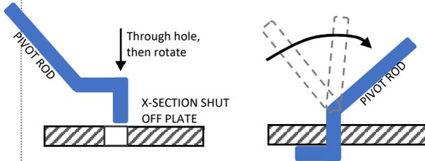
**Step 11:** Locate the PIVOT ROD bracket, insert the other end of the PIVOT ROD through the back of the PIVOT ROD BRACKET as shown (see below).
