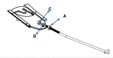
**Step 12:** Install HANDLE SHAFT to LOWER HANDLEs and PIVOT & BRACKET assembly as shown. Using 2" bolts and locknuts. **TIGHTEN BOLTS AND NUTS NOW.**
