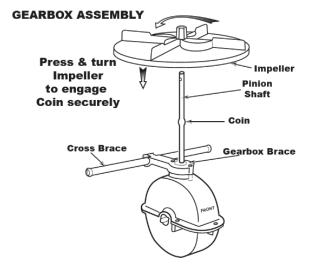
**Step 4:** Install GEARBOX by inserting the PINION SHAFT into hole in center of HOPPER bottom. The word "FRONT" on the GEARBOX must point to Front of the HOPPER.
