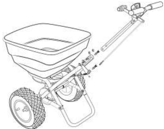
**Step 7:** Remove one 1/4-20 Hex Nut from the CONTROL ROD. Next, push LEVER forward to setting "0" to help align the CONTROL ROD with hole in PIVOT BRACKET, pull LEVER backward to insert CONTROL ROD through hole in PIVOT BRACKET. Now install 1/4-20 regular nut on to CONTROL ROD.
