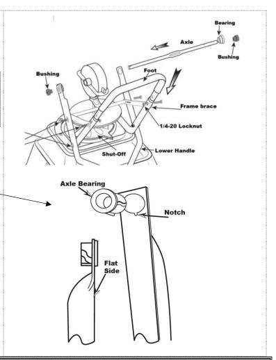
NOW GO BACK AND TIGHTEN ALL NUTS AND BOLTS STARTING WITH FIRST STEP. DO NOT OVER TIGHTEN.
